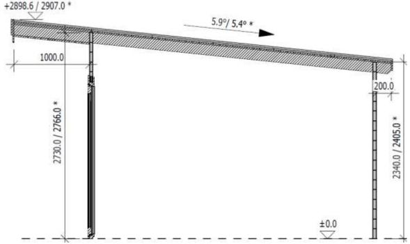
\*dimensions vary based on 45/80mm wall thickness
