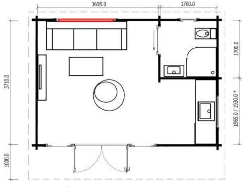
\*dimensions vary based on 45/80mm wall thickness
