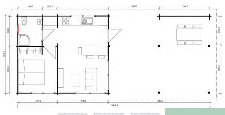
Customizable placement of windows marked red on the floor plan
