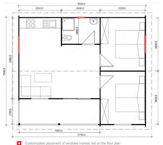
**LGL** LIVING ZONE Glulam timber 57 m<sup>2</sup> walls 80 VERANDA Wall thickness 10 m<sup>2</sup> mm TOTAL SIZE Floor plan can 67 m<sup>2</sup> be flipped
