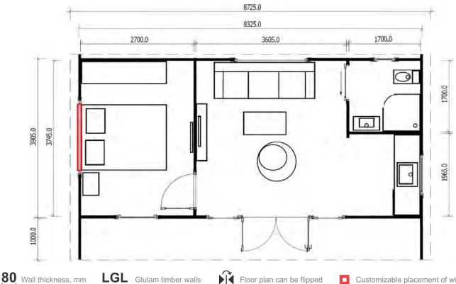
Customizable placement of windows marked red on the floor plan
